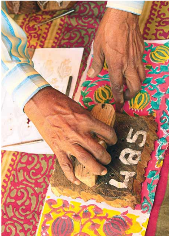
Checking registration of new wooden printing blocks; proof prints from new woodblocks (right)
